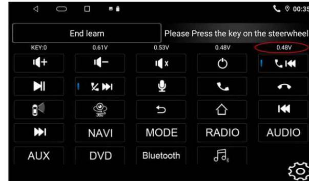
5. Press the icon
