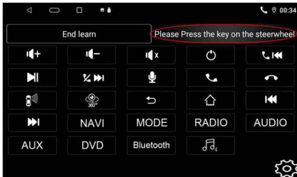
4. For example, press the pick up phone / last music button on the steering wheel. The voltage of the steering buttons will be displayed on the screen.
